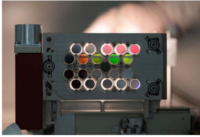
The Coronagraph Instrument (CGI) colour filter assembly.
