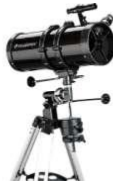
Celestron 6 inch Newtonian on an equatorial mount with manual slow motions
